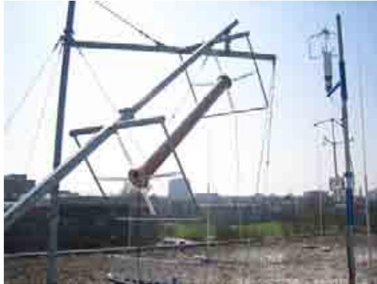
Figure 31: Rain-Wind induced vibrations experimental device
