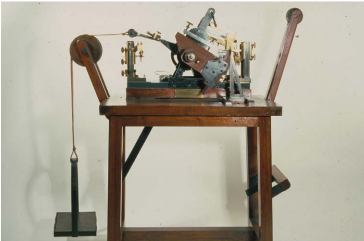
Fig. 2 – Bartoli-Felici switch, built in Florence, Italy by the Officine Turchini in 1894. The switch, from a design devised in 1874 ([F.50] in Felici's list of publications in the following) was aimed at fast opening/closing of circuits for induction experiments (University History Museum, University of Pavia).
