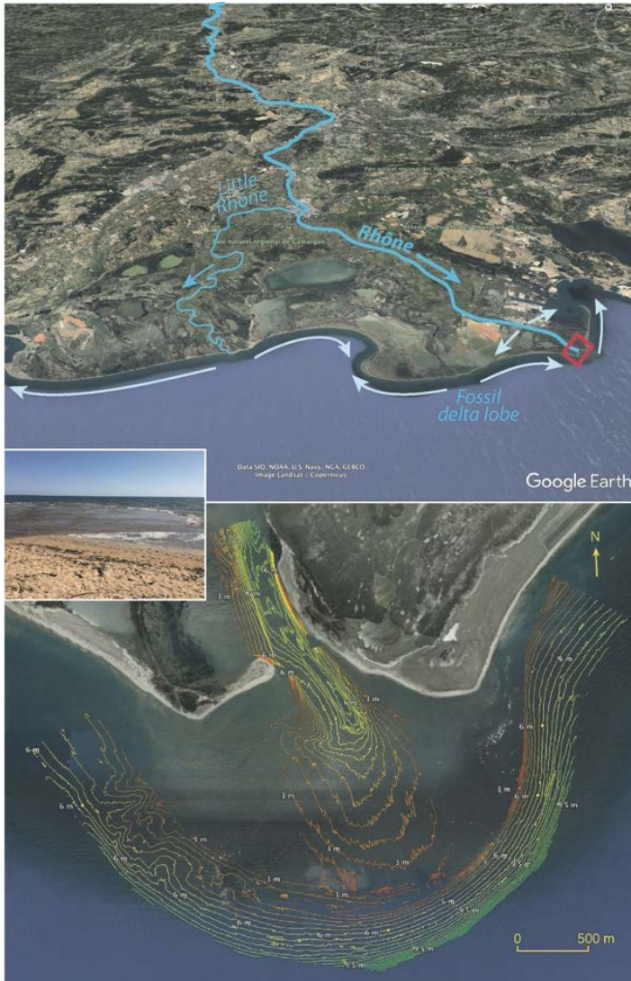
Figure 2 – River-to-coast sediment connectivity in the lower Rhône river and delta in France. Top image shows engineered sediment flux diversion to the advantage of the main Rhône distributary. Arrows show sediment (essentially fine-grained) spill-over onto the deltaic plain, and divergent (erosional sectors) and convergent (depositional sectors) bedload-transport sediment cells along the coast, including reworking of an abandoned delta lobe (from Sabatier and Anthony, 2015). Red box represents area of the river-mouth bar with bathymetry shown in bottom image. Photo insert on the left shows the small sandy river-mouth bar on the Argens delta, about 120 southeast of the Rhône delta.
