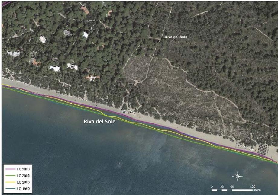
Figure 2 – Detail of the LC evolution at Riva del Sole.
