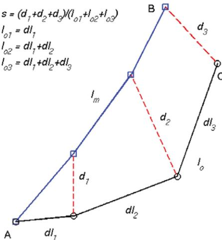
Figure 1 – Example showing the quantities involved in the calculation of the Skill Score Index, where  $l_o$  and  $l_m$  are the lengths of the observed and modelled paths, respectively. Source: [21].
