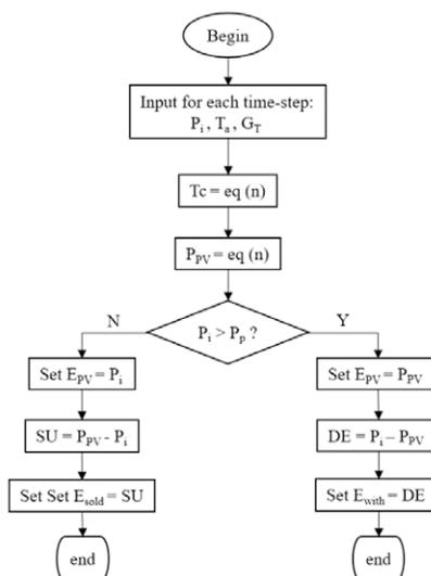
Figure 2 – Diagram flow of a photovoltaic scenario.
