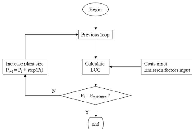
Figure 3 – Diagram flow of LCC loop.
