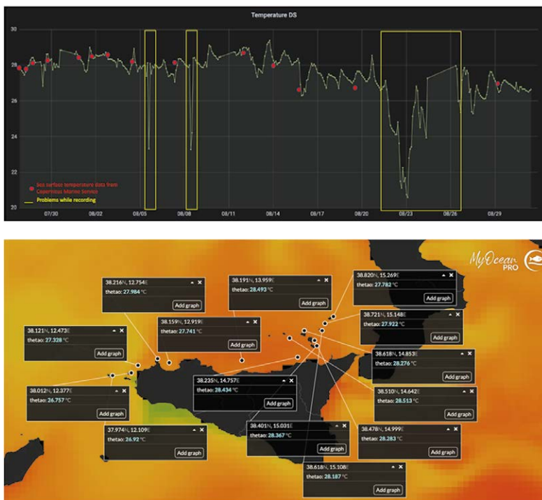
Figure 7 – (Upper) Graph of the temperature recorded by the system with comparison (Lower) with the sea surface temperature available from Copernicus Marine Service showing very good.
