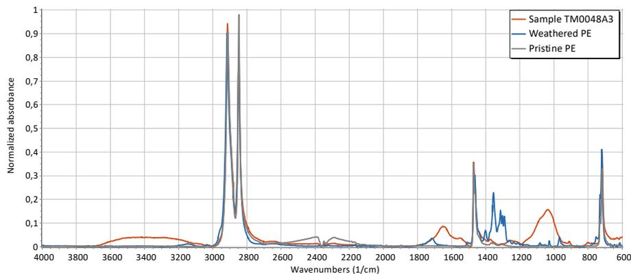
Figure 4 – Infrared spectra of pristine PE (gray), artificially UV-weathered PE (blue) and a PE microplastic from the Tara mission (TM0048A3) (orange). The band between 1100  $\text{cm}^{-1}$  and 1045  $\text{cm}^{-1}$  could reflect the presence of diatoms on the surface of TM0048A3.
