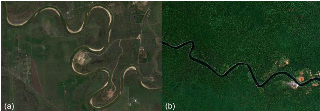
Figure 99. Typical behaviour of channel width in two meandering rivers. In (a) (Brazos River, Texas) the maximum widths are experienced at bend apices; in (b) (tributary of the Amazon River, Brazil) the minimum widths are found at bend apices and local widening is experienced in straight reaches (source Google Earth, courtesy of Rossella Luchi).
