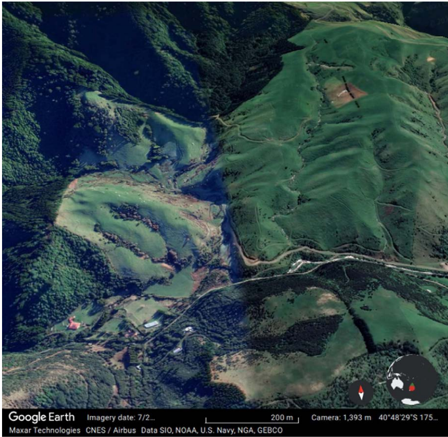
Figure 167. Google Earth image of a part of the Waipoua River catchment in the North Island of New Zealand, showing sub-catchments separated from the main stem by large steps in channel elevation.
