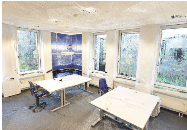
Fig. 6: Point cloud from terrestrial laser scanner of an office in the Building Inspector XR.
