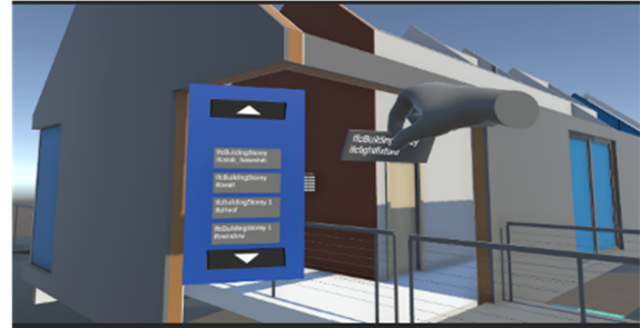
(b) Snapshot of the mapping between the work package and the reference model (virtual layout of the building).
