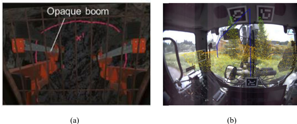
Fig. 1. (a) See-through visualization of the boom presented in (Aromaa et al., 2020) , (b) Visualization of the environment using point cloud presented in (Palonen et al., 2017)
