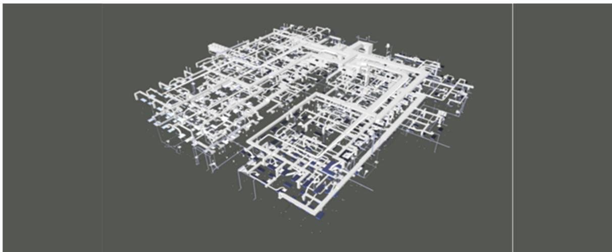
Fig. 7: Single discipline model- stand alone MEP Model of the Building (from US GSA BIM guide 07)
