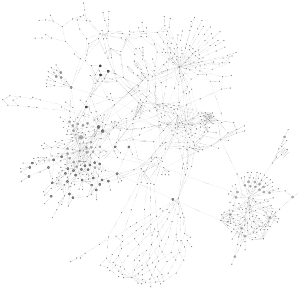
Fig. 5: Representation in the graph system of the geometric object (wall system) starting from IFC files
