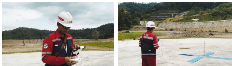
Figure 6. Digital Survey process with Drone Mapping
