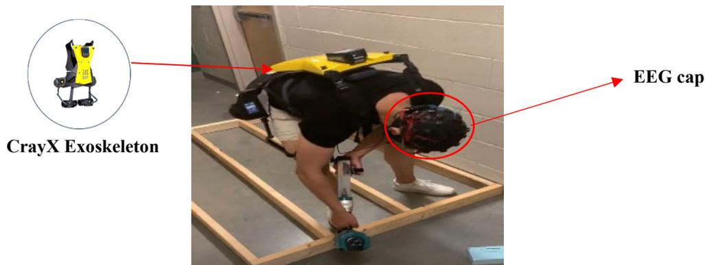
Fig. 3: Participant performing framing task while wearing an exoskeleton and EEG cap.
