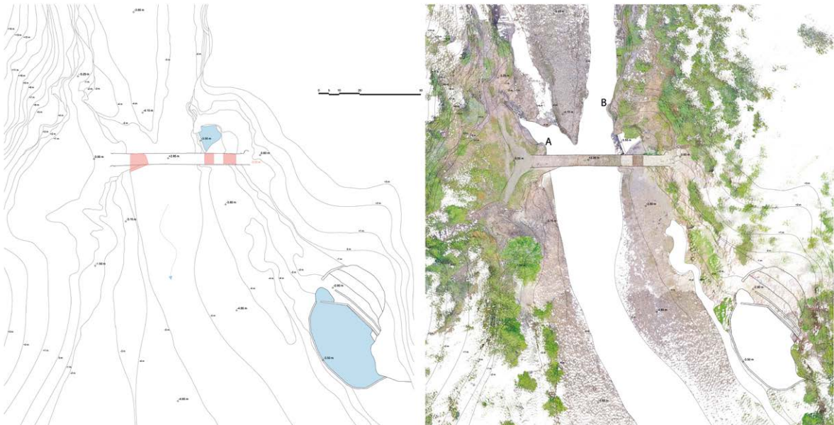
Figure 3.16 – Left, Plan of the Kadiu Bridge highlighting the piers (in orange), the contour lines of the area, and the thermal pools (in light blue). Right, plan view of the point cloud of the laser scanner survey, indicating the rock outcrops (A and B) protecting the bridge abutments.
