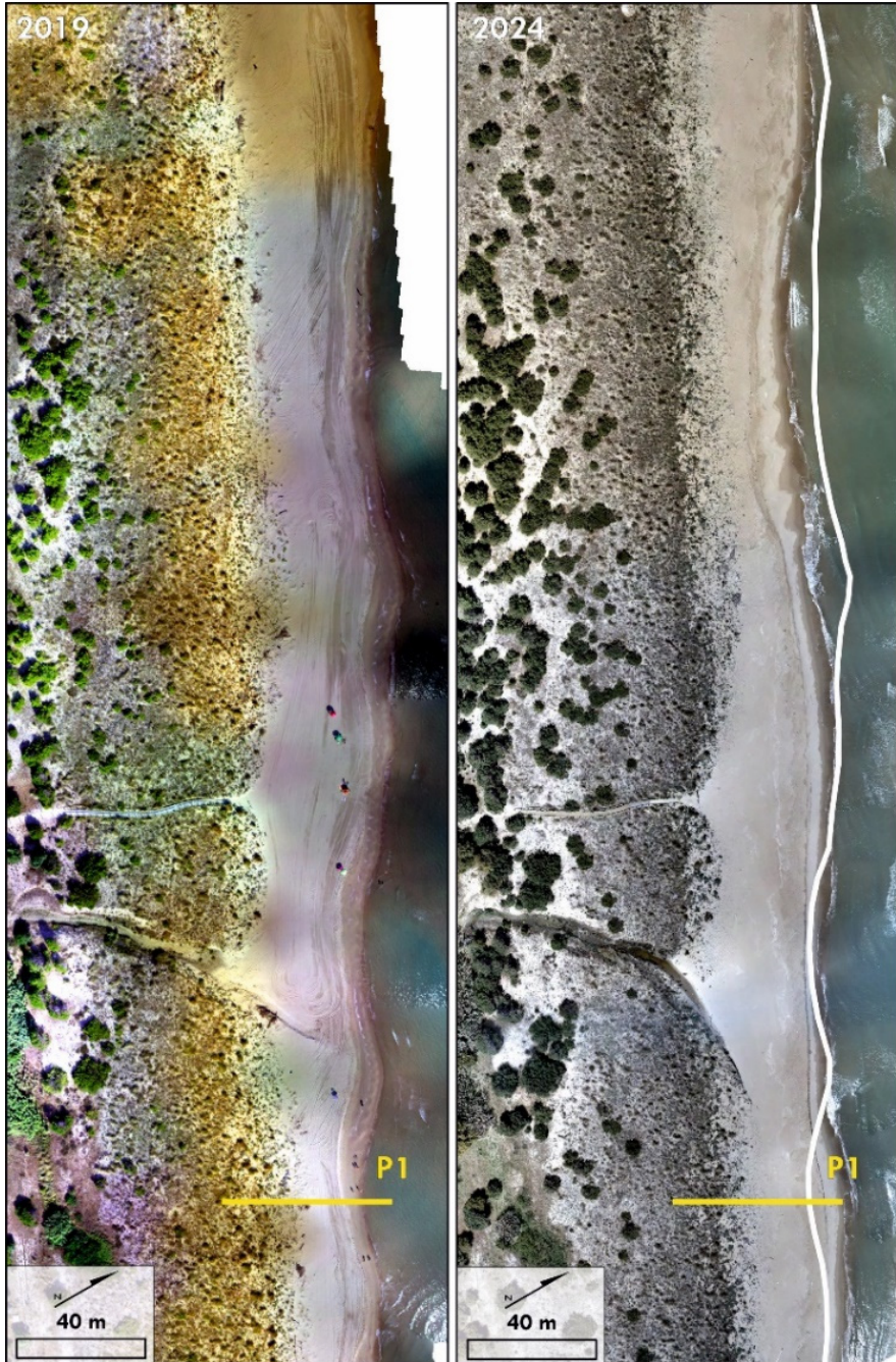
Figure 4 – Comparison between the orthophotos obtained elaborating drone surveys performed in 2019 and 2024 on the Petacciato beach. The 2019 UAV shoreline is marked in white.
