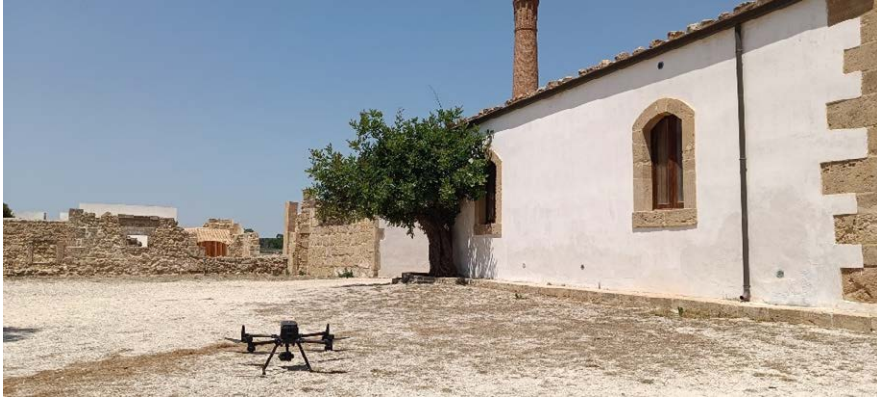
Figure 3 – Lidar survey phases by Drone Matrice 300.
