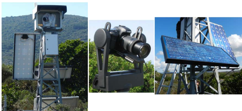
Figure 1 – Different view of APOS installed in the experimental site Capo Caccia, Italy: system mounted on the trellis with camera/robot inside the protection case (left), camera coupled to GigaPan robot (centre) and power supply system (right).
