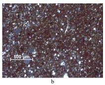
Figure 9 – Images at the optical microscope in thin section, crossed polarized light: bedding mortar with presence of serpentinite in the aggregate (a); brick with opaque groundmass and the almost absence of the framework (b).
