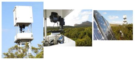
Figure 3 – Different view of PHATOS installed in the experimental site Capo Caccia, Italy: system mounted on the trellis with camera/robot inside the protection case (left), camera coupled to Rodeon robotic arm (centre) and power supply system (right).
