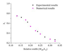
Figure 6 – Comparison between numerical results of  $k_t$  obtained via the NWT and experimental measurements from Liang et al. [3] ( $W_{FB}$ =0.5 m,  $D_{FB}$ =0.16 m,  $W_{FB}/L_w$ =0.13÷0.33,  $H_i$ =0.07 m and  $d_w$ =0.6 m)
