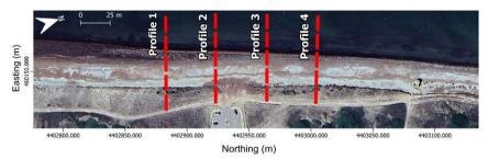
Figure 4 – The four cross-shore profiles were located using the RTK-DGPS in all the field campaigns. Geographical coordinates are in the WGS84/UTM zone 32N system (EPSG:32632).
