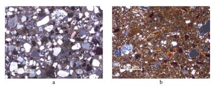
Figure 10 – Images at the optical microscope in thin section, crossed polarized light: bedding mortar with an abundant aggregate (a); brick with a weakly birefringent groundmass and abundant framework consisting of quartz and feldspars (b).
