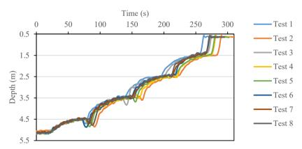
Figure 4 – Depth evolution for 4.5, 3.5, 2.5, and 1.5 meters, remaining at each setpoint within the error range for 20 seconds.
