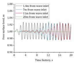
Figure 4 – Time histories of the free surface levels at different NWF sections (1.4 m, 7 m, 11 m and 20 m far from wave inlet).
