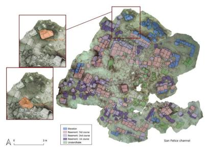
Figure 6 – Orthophoto from photogrammetric survey and digitization in GIS of the basement and wall of the San Felice well-cistern. In the rectangular sections, the movement of the corner of the wall from July to September is evident (elaboration: authors).
