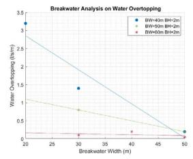
Figure 3 – Breakwater Analysis on Water Overtopping.
