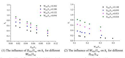
Figure 8 – The influence of the BDB's design parameters on  $k_t$  under the 100-year return period wave condition ( $H_i$ =0.043 m,  $T_p$ =1.0 s,  $D_{FB}$ =19÷206 mm and  $W_{FB}$ =25÷550 mm).
