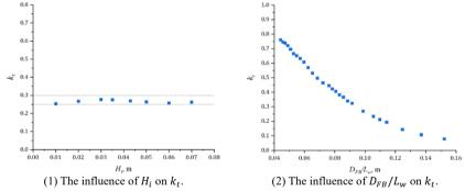
Figure 7 – The influence of  $H_i$  and  $L_w$  on the  $k_t$  of deep-draft fixed BDB ( $H_i$ =0.01~0.07 m,  $L_w$ =0.9~3.1 m,  $D_{FB}$ =206 mm and  $W_{FB}$ =471 mm).
