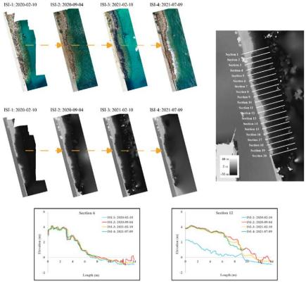
Figure 4 – Extracting information regarding armor units' displacement for the rubble mound structure of the domestic ferry and cruise domain in Lavrio port [19]. The elevation profiles were constructed based on the DEMs generated in Step 1 of Figure 1.
