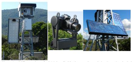
Figure 1 – Different view of APOS installed in the experimental site Capo Caccia, Italy: system mounted on the trellis with camera/robot inside the protection case (left), camera coupled to GigaPan robot (centre) and power supply system (right).
