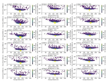
Figure 5 – Average distance between Control Point and Checkpoint Root Mean Square Errors (RMSE).
