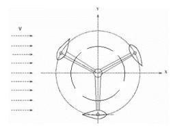
Figure 2 – Three bladed VAWT schematic.
