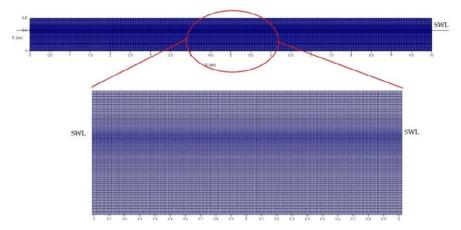
Figure 2 – The general view of the grid and zoom of the grid in the vicinity of the water surface.
