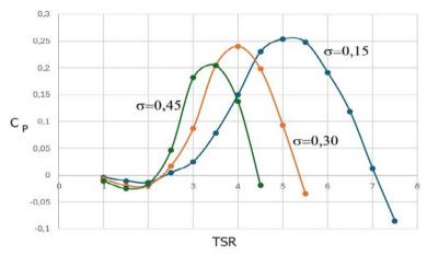
Figure 1 – Power coefficient (*CP*) vs. tip speed ratio (TSR) for 3 bladed VAWTs for different solidity values ( $\sigma$ =Nc/R).
