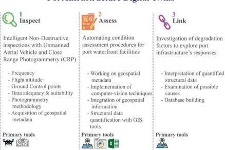
Figure 1 – The steps of a SHM-based DT guide for port waterfront facilities.
