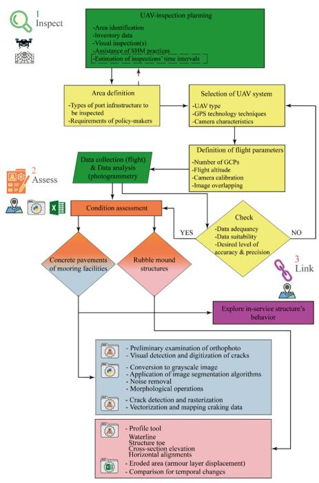
Figure 2 – The DT architecture for port waterfront facilities.
