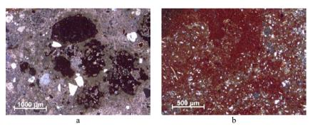
Figure 7 – Images at the optical microscope in thin section, crossed polarized light: bedding mortar of the bastion with presence of pozzolan (a); brick with opaque groundmass and almost absence of framework (b).
