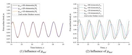
Figure 5 – Influence of the mesh resolutions on the free surface wav emotion measured at WG-b located 7 m far from the wave inlet.
