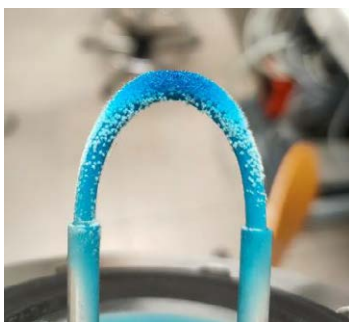
Figure 5.19. Photograph of [\text{VO}(\text{acac})_2] crystals formed during condensation of sublimed fraction on the cold finger.
