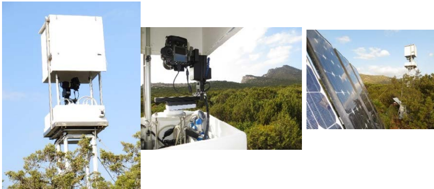
Figure 3 – Different view of PHATOS installed in the experimental site Capo Caccia, Italy: system mounted on the trellis with camera/robot inside the protection case (left), camera coupled to Rodeon robotic arm (centre) and power supply system (right).
