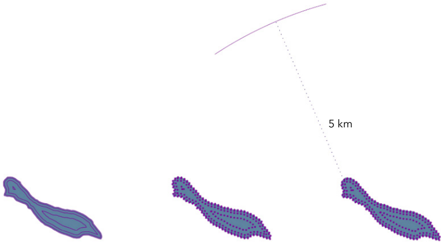
Figure 4 – Outline of the wetland discretization process and definition of the maximum visual field extension.
