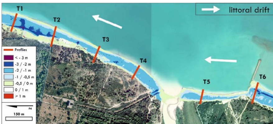
Figure 3 – Location of the topographical profiles (T1-T6) extracted from DEMs and differences in topographical height estimated from the comparison between DEMs relative to the years 2023 and 2013.
