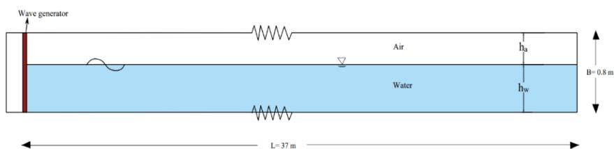
Figure 1 – Sketch of wave flume (not to scale). Overview of the simulation setup following the physical experiments, where  $h_w$  and  $h_a$ , represent the water depth and height of the air region, respectively.  $L$  and  $B$  are the length and height of the flume, respectively.
