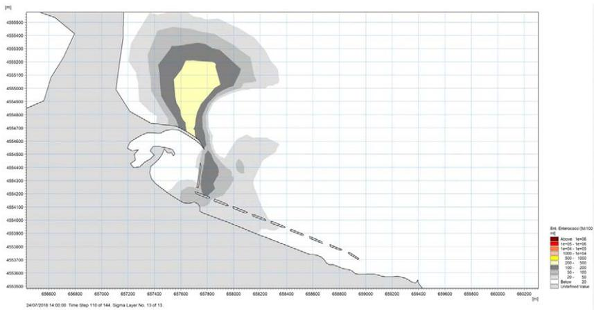
Figure 11 – Bacterial concentration plume at about 14.00 a.m. on July 24<sup>th</sup>, 2018 (15 hours after the opening of the sluice gates).
