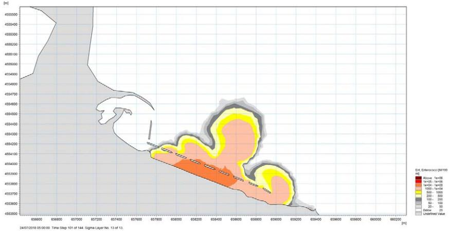
Figure 8 – Bacterial concentration plume at about 05.00 a.m. on July 24<sup>th</sup>, 2018 (6 hours after the opening of the sluice gates).
