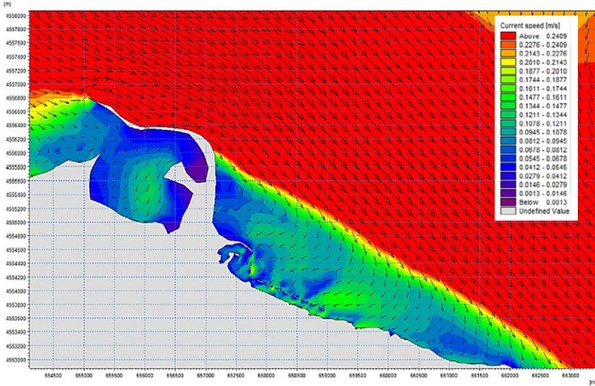
Figure 5 – Sea surface currents circulation on the July 24<sup>th</sup>, 2018, at 10.00 a.m. (after three days of computing).
