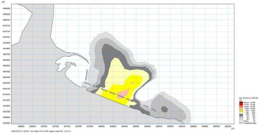
Figure 10 – Bacterial concentration plume at about 11.00 a.m. on July 24<sup>th</sup>, 2018 (12 hours after the opening of the sluice gates).
