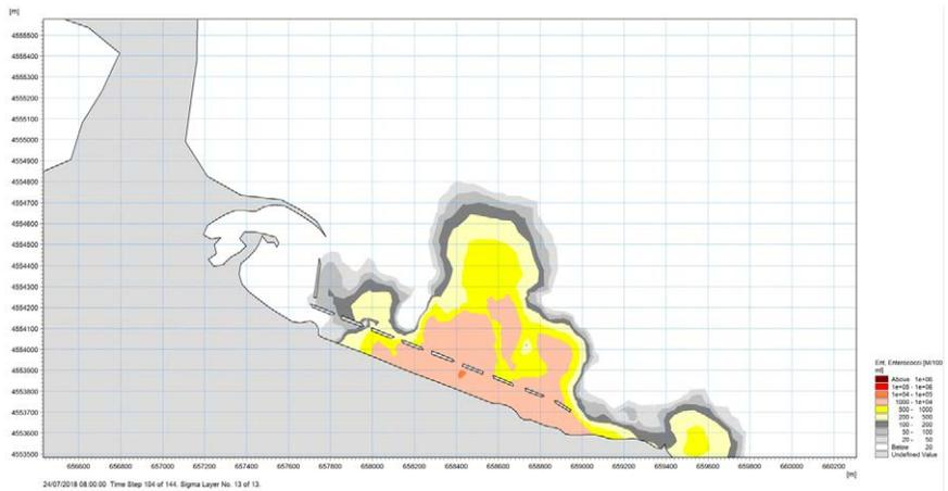
Figure 9 – Bacterial concentration plume at about 08.00 a.m. on July 24<sup>th</sup>, 2018 (9 hours after the opening of the sluice gates).
