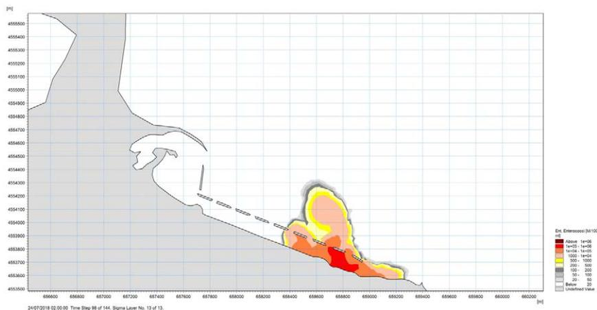
Figure 7 – Bacterial concentration plume at about 02.00 a.m. on July 24<sup>th</sup>, 2018 (3 hours after the opening of the sluice gates).
