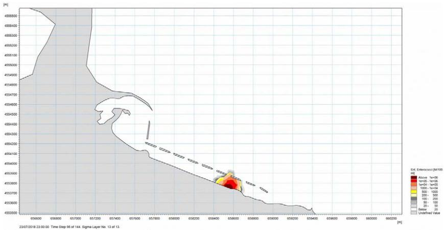
Figure 6 – Bacterial concentration plume at about 11.00 p.m. on July 23<sup>rd</sup>, 2018.
