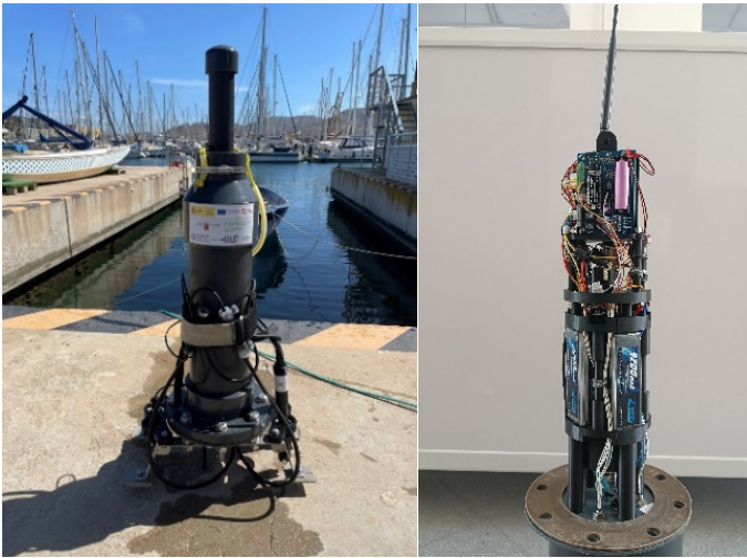
Figure 2 – External and internal architecture of the \mu -Nautilus profiler.
