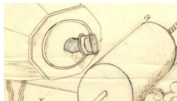
Fig. 3 Enlargement of Scott's original drawing, showing how, at the end of the acoustic horn, the membrane to which the boar's hair is attached is slightly offset from the axis of the horn, in order to allow for optimal vibration inscription on the rotating cylinder.
