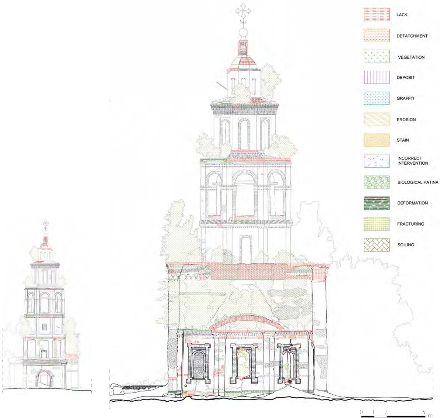
Fig. 10 Decay analysis on Rubezhskaya church Mapping of the main degradations revealed by the 2018 survey, preparatory to the definition of a restoration intervention strategy.
