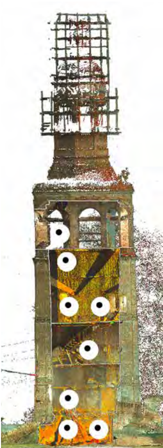
↓ Fig. 08 Scan of the Bell tower View of the scans position inside the tower. This image is the result of data registration between interior and exterior part of the building.
