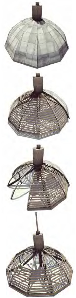
Fig. 11 Structural analysis of Bondyug Church the building is constructed almost entirely as a traditional timber-frame structure. Using advanced 3D modelling techniques, a virtual reconstruction of the roof assembly has been developed, allowing the hypothesised geometry, joinery details and load-bearing behaviour of the original covering system to be studied and visualised.
