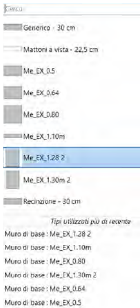
Fig. 12 Structuring of masonry walls It was carried out on the basis of the point cloud data. Starting from a generic wall family, the walls were then characterised as specific model components and renamed according to an internal project coding system.
