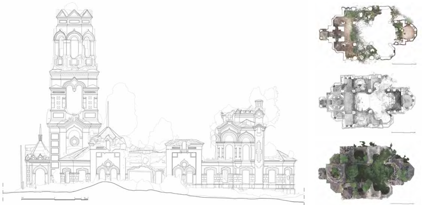
↑ Fig.08 2D drawing elaborated from point clouds by TLS and UAVs Vectorial and materic plans and ections of Blagoveshchenskaya Church.
