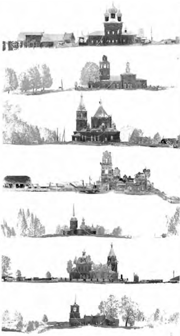
Fig.09 Global archive of ScanWorlds for different sites in Upper Kama survey documentation Point clouds strategy of acquisition as considered the different availability of access to monument's space (interiors and exteriors inside the fences) and the complexity of surrounding environment (alone standing in the forest or in the middle of villages and cities).
