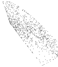
Figura 42. Point cloud sampled from the model of a ship hull.
