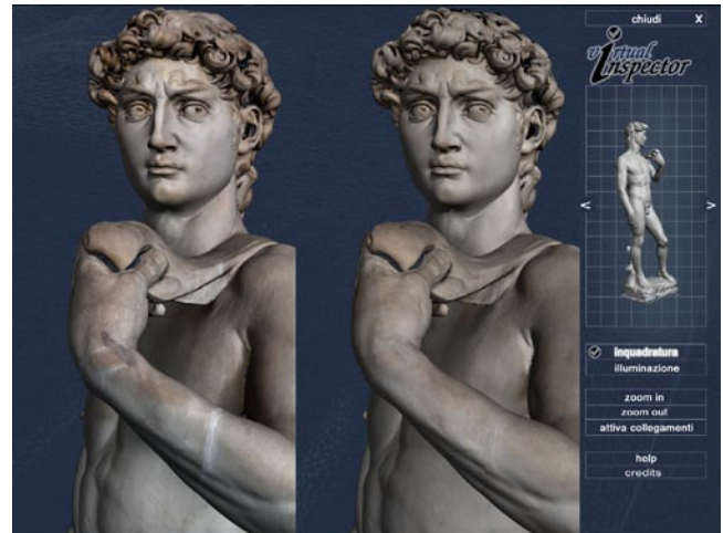
Figure 3: Two set of around 60 images each (depicting the pre- and post-restoration status) have been mapped onto the digital model of Michelangelo's David and rendered in real time using the Virtual Inspector system. Digital model courtesy of Stanford University (Digital Michelangelo Project) and Museo Gallerie dell'Accademia, Florence.
