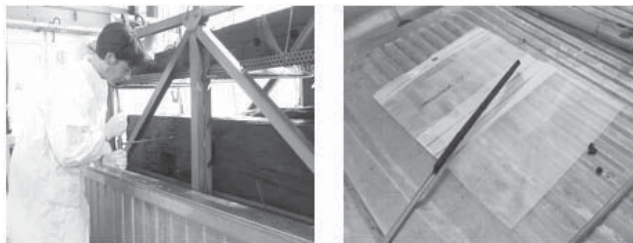
Fig. 1. Drilling in the wood timber and the obtained core sampling.
