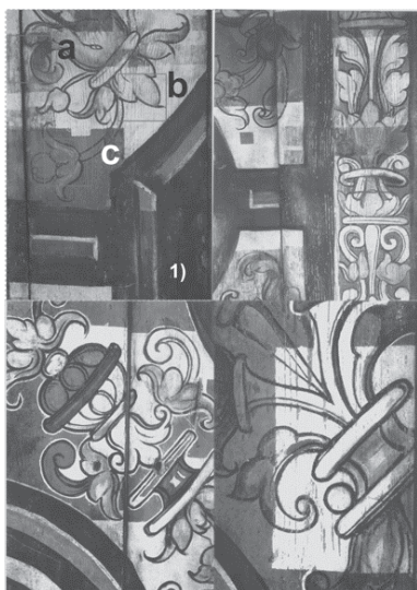
Fig. 4. Laser cleaning tests. Photo 1) shows comparison of removal of secondary encrustations from a polychrome: a) chemical agents, b) laser, and c) original surface.
