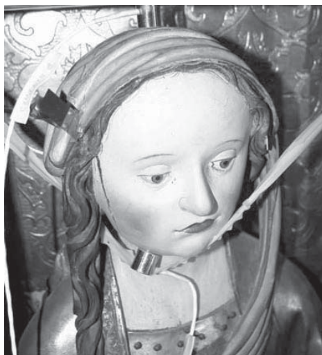
Fig. 5. AE sensors coupled to the statue's head during on-site monitoring of the wooden altarpiece.
