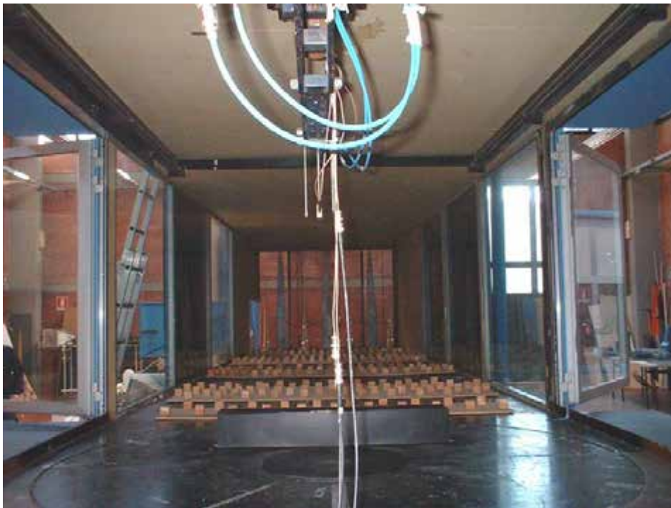
Figure 5.5 Experimental setup with prism in the CRIACIV wind tunnel
