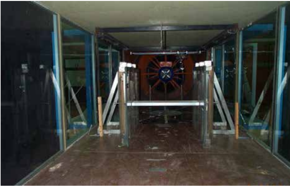
Figure 2.1 Aeroelastic section model in the CRIACIV boundary layer wind tunnel
