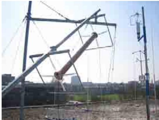
Figure 31: Rain-Wind induced vibrations experimental device
