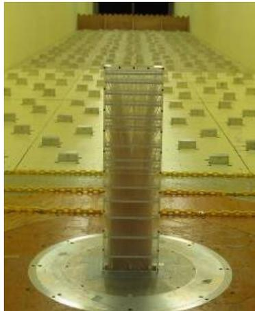
Figure 1: Pressure-tapped benchmark building model inside wind tunnel.
