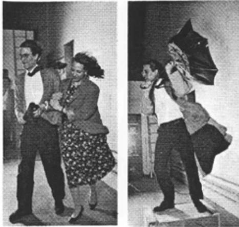
Figure 6: wind tunnel exposure of people at 70 km/h winds.
