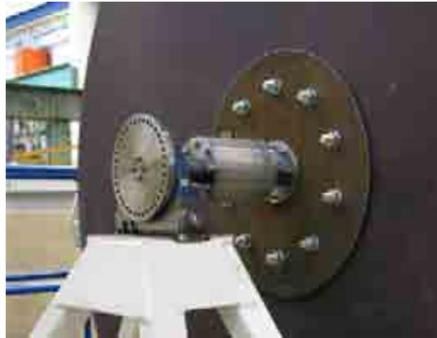
Figure 2 Turntable and force transducer configuration
