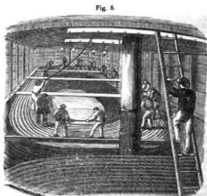
**Figura 5.** Posa dei cavi sottomarini, trasportati nella stiva di apposite navi (T.P. Shaffner, *The Electric Manual: a Complete History and Description of the Semaphore, Electric and Magnetic Telegraphs of Europe, Asia, Africa and America, Ancient and Modern*, New York, 1859).
