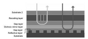
Fig.3 - Cross section of an HVD
