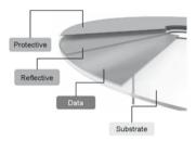
Fig.1 - Cross section of an optical disc
