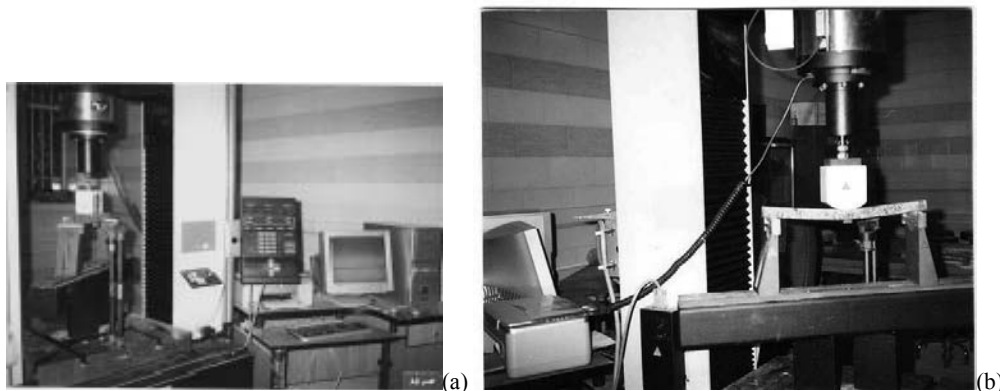
Fig. 2 – Static bending test assembly. (a) Testing apparatus, (b) sample assembly and loading
