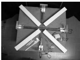
Fig. 17 – The “deformometric kit”, purposely designed and built for monitoring this kind of shields. Four Plexiglas feelers slide freely on perpendicular low friction rails.
