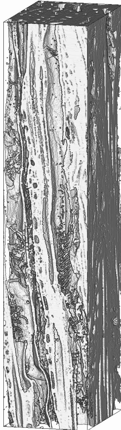
Fig. 2. A typical 3D view of the sample from Sesin-bosatsu-rituzou, registered national treasure, curved by UNKEI in Kamakura period, obtained at BL20XU, SPring-8. Wood is identified as Katsura ( Cercidiphyllum japonicum )
