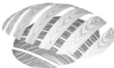
Fig. 2 – Two perpendicular cross-sections of the shield, obtained by Computed Tomography: the upper CT scan is on the smaller (“horizontal”) diameter, whereas the lower CT scan is on the larger (“vertical”) diameter. Drawings placed under CT scans put into evidence the longitudinal and transversal cross-sections of lamellae, and the random orientation of growth rings.
