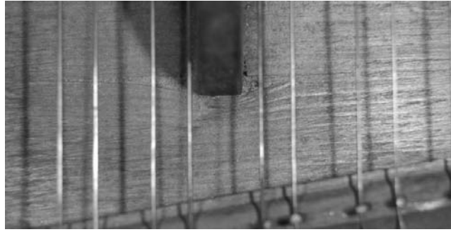
Fig. 6. Plastic deformations in pin block.
