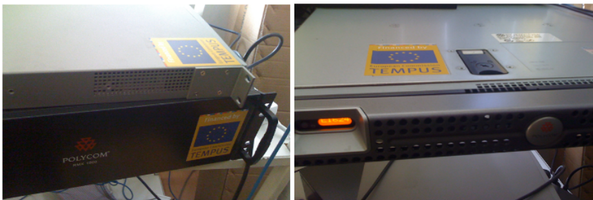
Figure 2. On the left the Polycom RMX 1000 and Polycom RSS 200 server, on the right the Polycom CMA 4000 server
