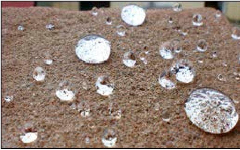
3. Effetto del rivestimento nanotecnologico su superficie porosa (foto Paola Borgarello) 3. Effect of the nanotechnological coating on a porous surface (photo Paola Borgarello)
