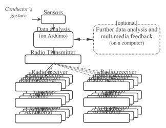
Figure 1. Overall system architecture design.
