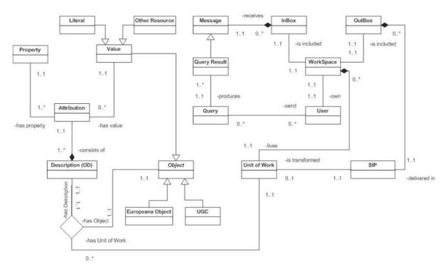
Figure 1 UML class diagram of the UGC service conceptual model
