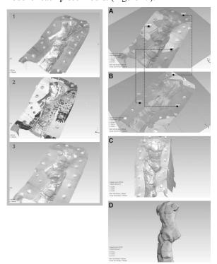
Figure 1. On the left: 1: initial alignment based on homologous points directly identified on the surface. 2: ine registration based on an I.C.P. (interactive closet point) algorithm. 3: Complete 3D digital model of a one piece-mould.On the right: A-B: tie points used to align the two piece-mould related to Giant's bust. C: concave side of the piece-mold. D: Complete 3D digital model of the Giant's bust.
