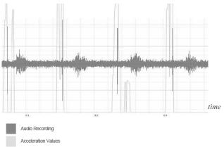
Figure 2. A comparison of the recorded voice audio and the recorded sensor data to measure their timing differences.
