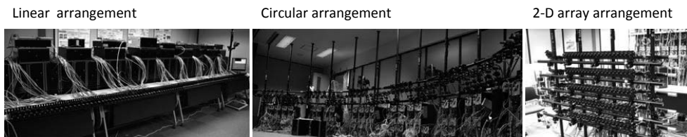
Fig. 1. 100-camera capturing system.
