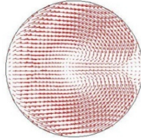
Fig.11: Fluid flow pattern in x-y plane, z=8.6 cm, at 270^0 ATDC, k-\varepsilon
