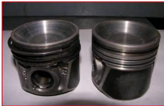
Fig.2 Modified pistons with enlarged bowl
