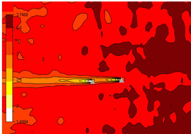
Fig. 6. Calculated wind field (Speed 2D) at the turbine's hub height (65 m a.g.l.) for the 90° sector in neutral condition.
