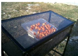
Fig 5a. Open sky solar dryer
