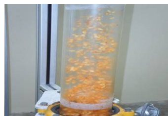
Fig.5b. Fluidized bed dryer
