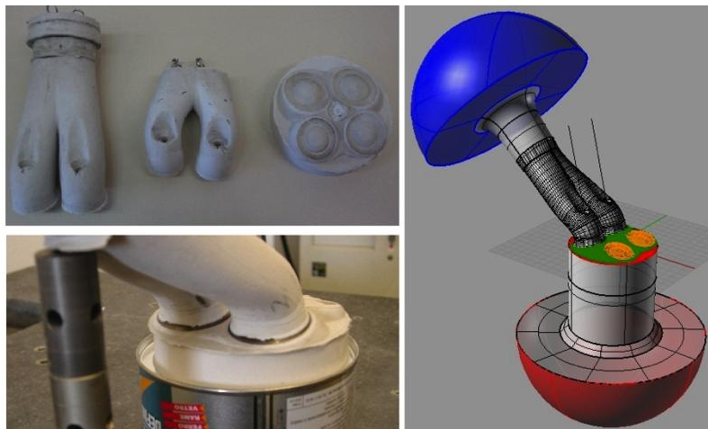
Fig. 7. Reverse engineering of Aprilia RSV1000 cylinder geometry: “rubber” cores of combustion chamber and manifolds (upper left); intake system assembly to be 3D scanned (lower left); reconstructed CAD surface of the whole intake system CFD domain (right).
