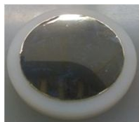
Fig. 7: Our manufactured reflective thin film
