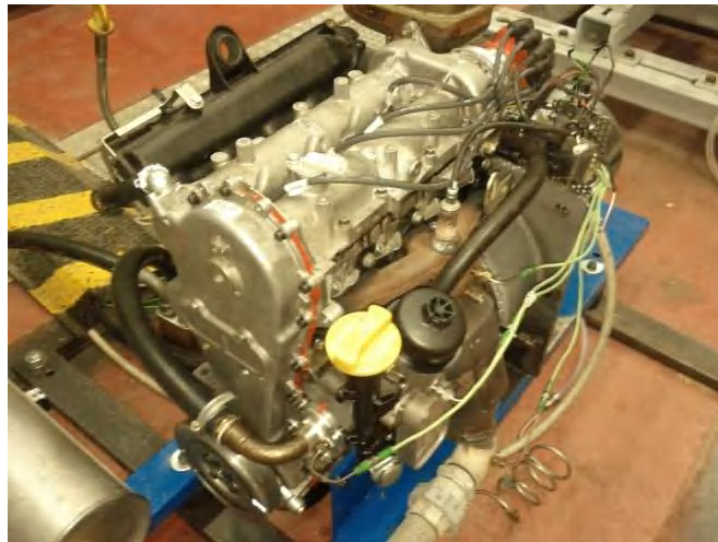
Fig.10: The 10 kW power unit during endurance test
