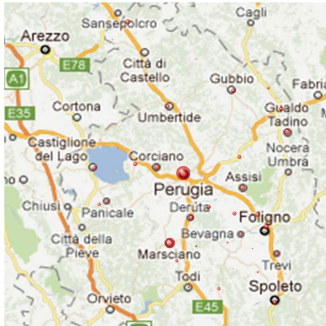
Figure 4: Bubble representation of the generated energy per year in Perugia province: the size of the spheres is proportional to the produced photovoltaic energy. To make a comparison among different bubbles, the energy that is yearly produced in Perugia municipality is 27,116.9 MWh/y; a complete numerical data-table for all the municipalities of the province is available in Appendix (see Appendix A, Table A.2).
