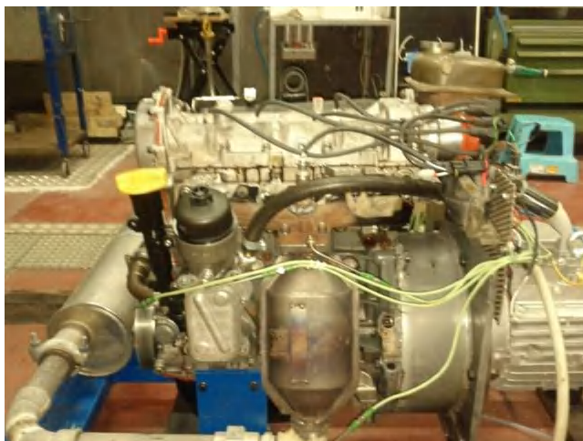
Fig.5 The prototype with catalyst and double oxygen sensor
