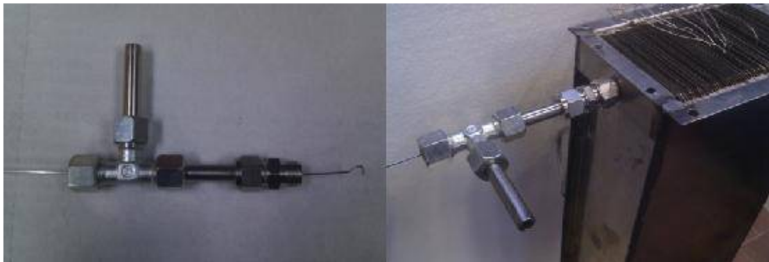
Fig 3: The static pressure probe (left) and the CPHE reformer stack (right).
