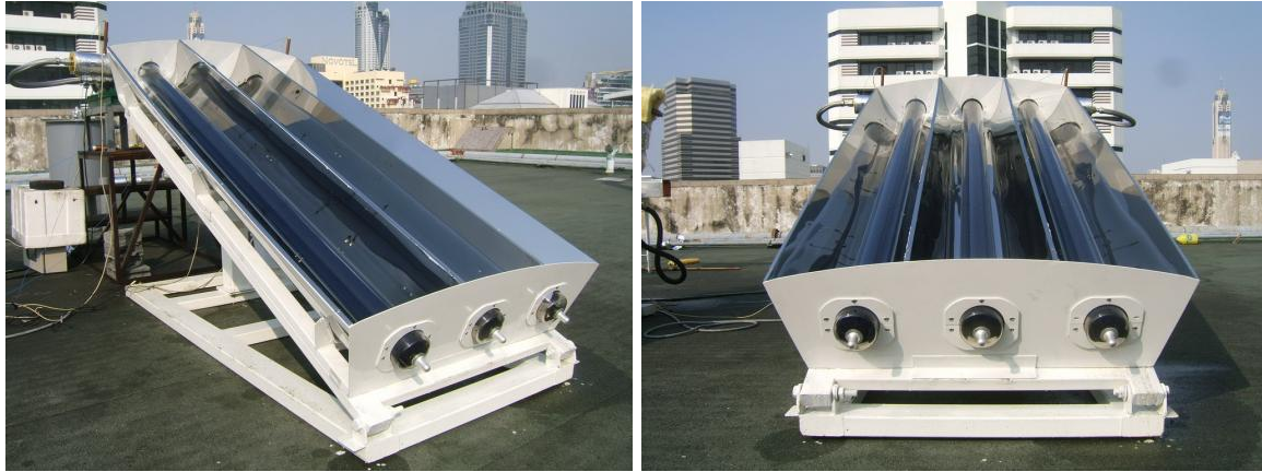
Fig. 6. The novel non-tracking solar collector has an overall width of 1 m and a length of 1.9 m.
