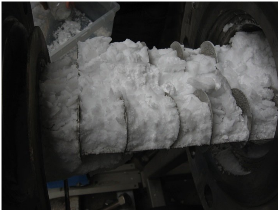
Fig. 6. Carbon dioxide hydrates on the internal heat exchanger.
