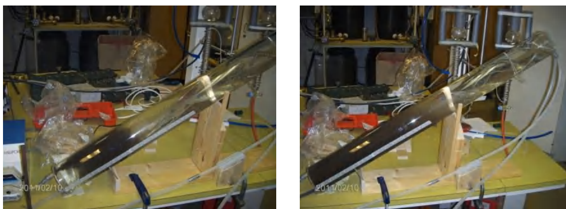
Fig. 7. A 30° inclined settling tube 0 minutes (left) and 2 minutes (right) from the start of the test.
