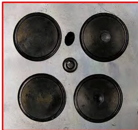
Fig. 3 Four valve head with spark plug
