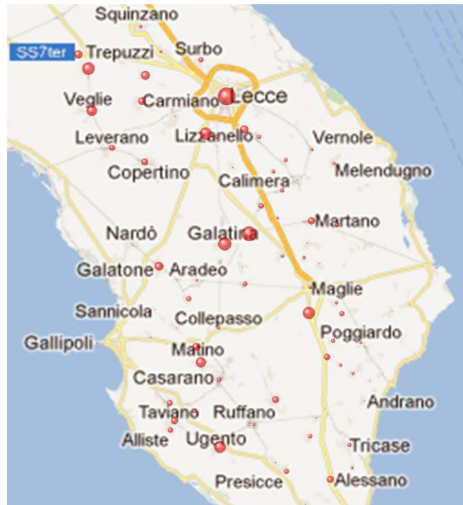
Figure 5: Bubble representation of the generated energy per year in Lecce province: the size of the spheres is proportional to the produced photovoltaic energy. To make a comparison among different bubbles, the energy that is yearly produced in Lecce municipality is 42,566.5 MWh/y; a complete numerical data-table for all the municipalities of the province is available in Appendix (see Appendix A, Table A.3).
