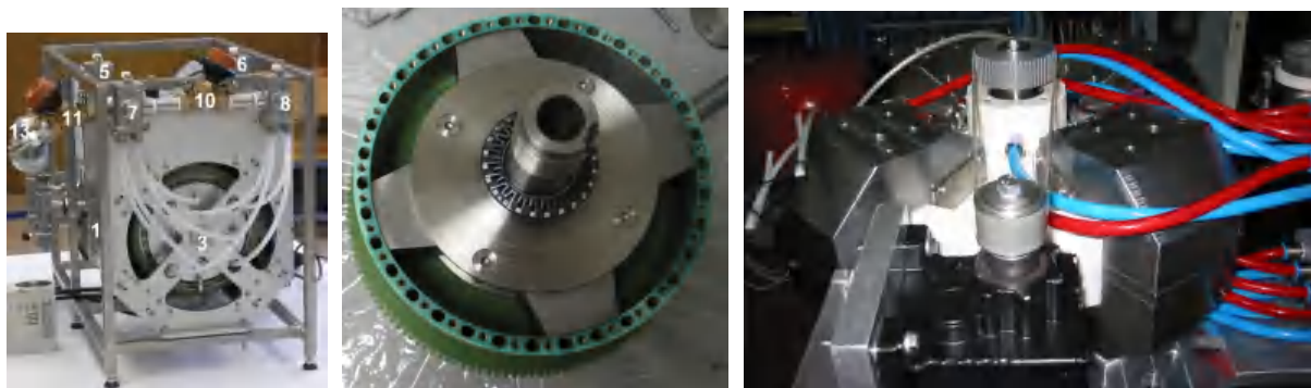
Figure 3: Left: The first rotary magnetic refrigerator built at the University of Ljubljana. In the middle, the coaxial ring is shown with 34 magnetocaloric regenerators[54]. Right: second rotary magnetic refrigerator built at the University of Ljubljana.
