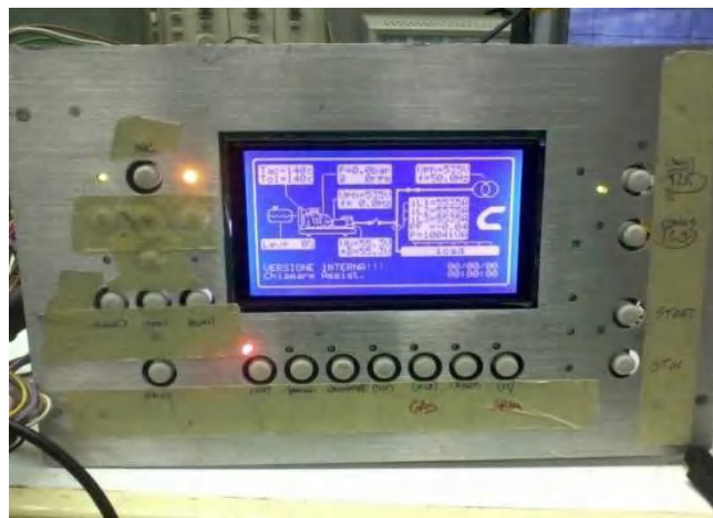
Fig. 4 Prototype cogenerator control/management system
