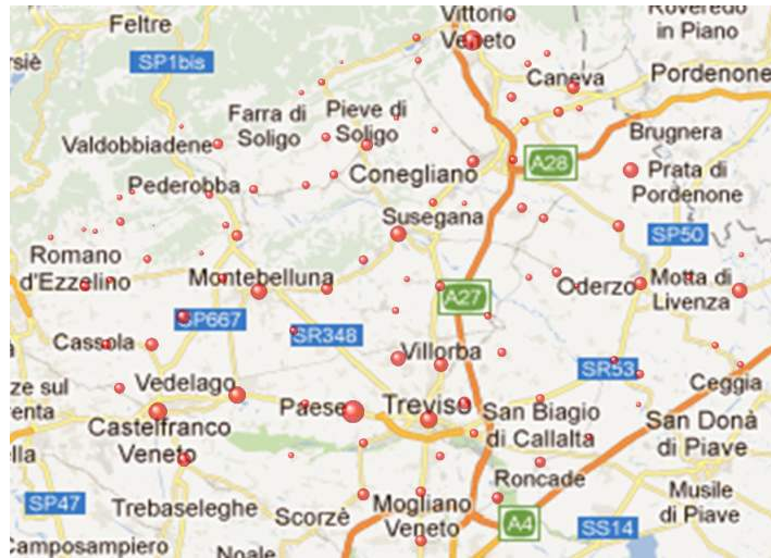
Figure 3: Bubble representation of the generated energy per year in Treviso province: the size of the spheres is proportional to the produced photovoltaic energy. To make a comparison among the size of different bubbles, the energy that is yearly produced in Treviso municipality is 3,320.2 MWh/y; a complete numerical data-table for all the municipalities of the province is available in Appendix (see Appendix A, Table A.1).
