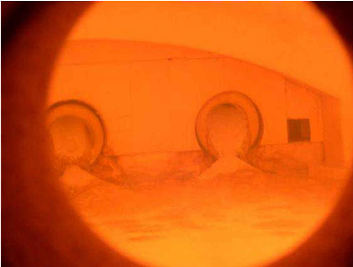
Figure 10: View into the GlasFLOX glass melting furnace
