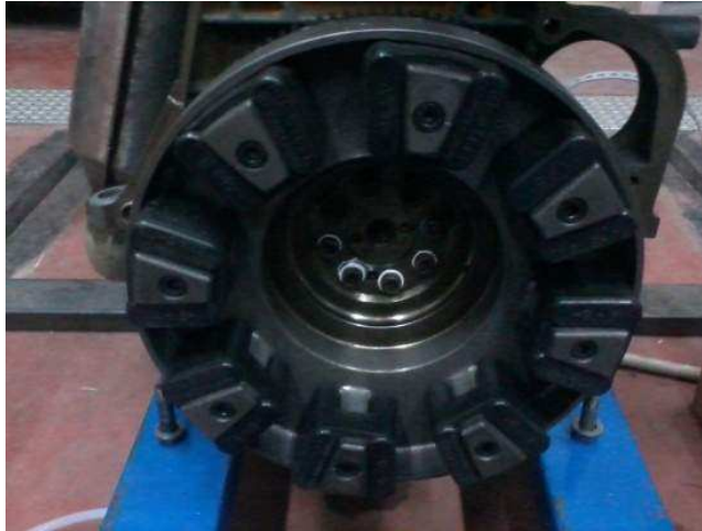
Fig.9 Elastic coupling with high inertia flywheel
