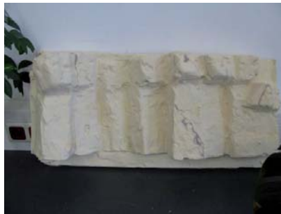
Figure 7: Detail of the passion, death and resurrection of Jesus Christ, CNC milled in model material
