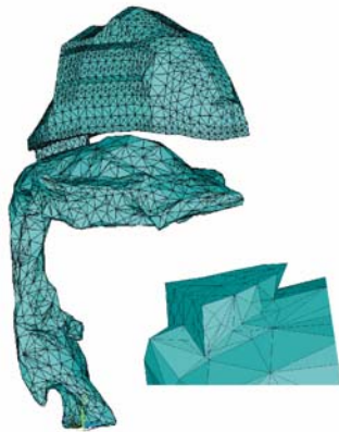
Fig. 1 FE model of the supraglottal spaces for vowel /a/ with the nasal cavity joint by cleft model.
