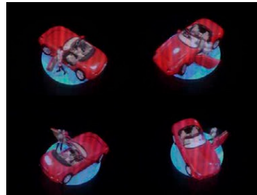
Fig. 7. Displayed images of Holo-Table in different directions.
