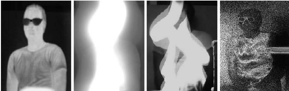
Figure 3.34: Imaging of an alive human being seen through two stoves flames. From left to right, thermographic image without flames, thermographic image with flames, visible image with flames, holographic reconstructed image with flames.
