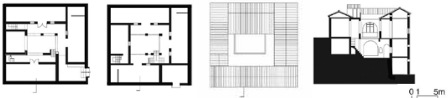
Fig. 2 Plans and section of a typical islamic courtyard house in Chefchaouen, Morocco (drawings: L. Dipasquale)
