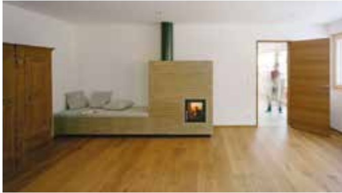
Fig. 8-9 Rammed earth stove, developed by Martin Rauch (© Lehmo).
