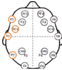
Figure 2: Location of the electrodes in the Emotiv EPOC kit. The channels corresponding to Geschwind-Wernicke model are marked with orange.
