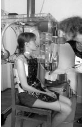
Fig 1. The EMA technician is attaching the coil sensors to the subject.
