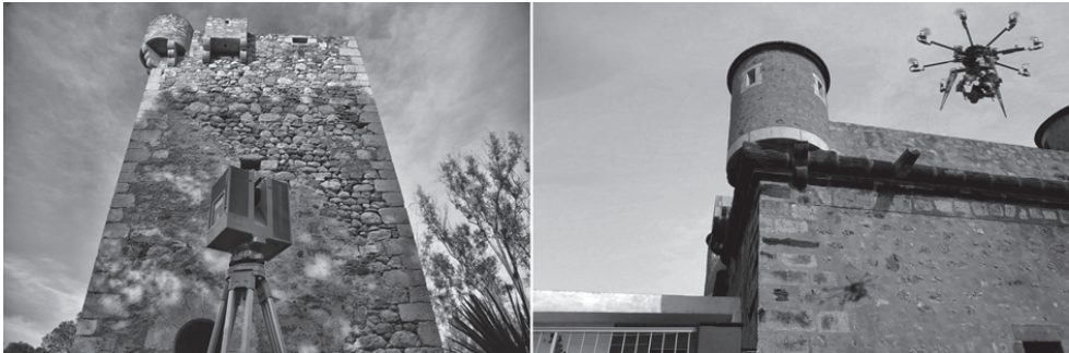
Fig. 3 - 3D Laser Scanner and Octacopter Drone at work (G. Verdiani, S. Giraudeau)
