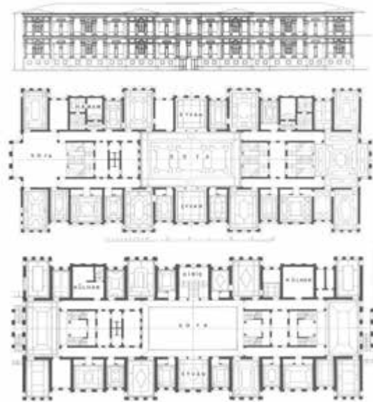
The reconstruction of the Çifte Palaces before the fill in of the atrium. Below, the original plan of the twin palaces
