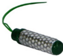
Figure 13.15: Soil water potential sensor for agrometeorological use (example: Watermark), (Source: Pacher).
